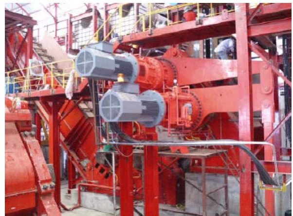
図2 モータ駆動砂糖キビ圧搾機外観 Fig.2 Motor Drive Pressure Feeder for Mill
