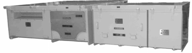
1C2M制御用VVVF装置 (VVVF+断流器)
