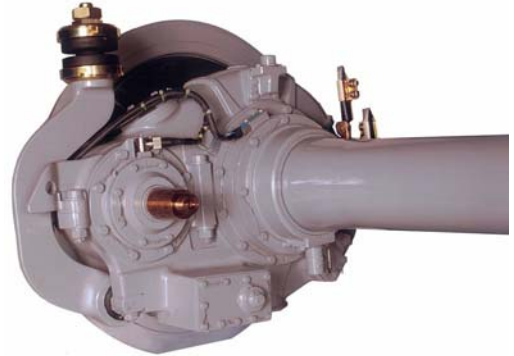
図2 駆動装置 Fig.2 Driving gear unit
