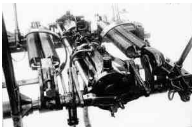
図12 G形パンタグラフ台枠搭載機器 Fig.12 Mounted equipments on type G pantograph base
