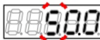
Acceleration time changed to "50.0" sec
