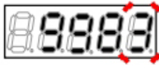
Specify "9983" if the measured value is 9.983 V
