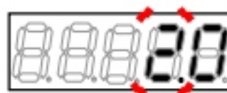
Forward_JOG_frequency changed to "2.0" Hz in [V/f]
