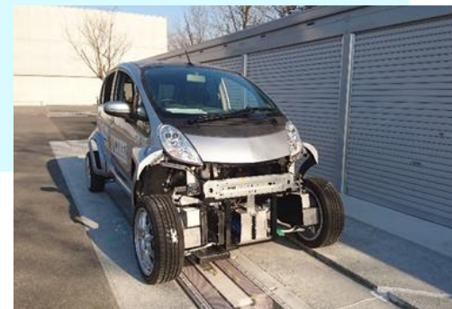
Research and development on wireless power supply while driving.
