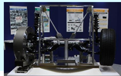
Development of flat-type dynamo for automatic operation vehicle evaluation.
