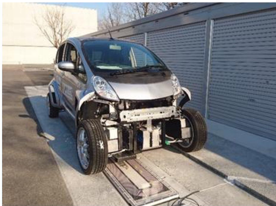
Wireless in-wheel motor (Unit No.2)
