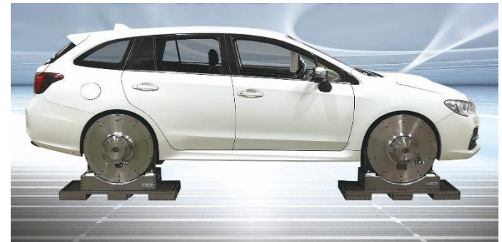
Actual vehicle tests with In-Tyre-House dynamo
