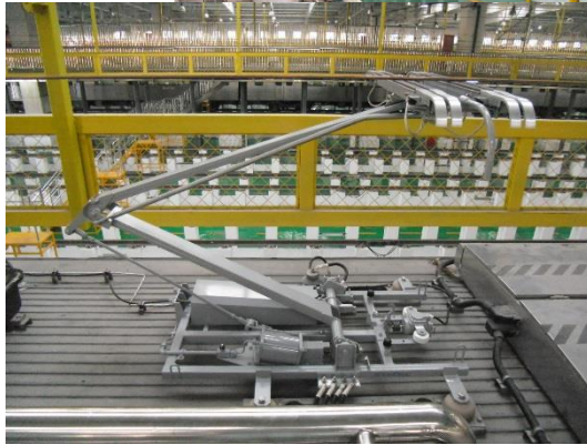
Test pantograph mounted on Line 6 of Beijing Subway
