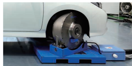
ITHD enables tests that include steering
