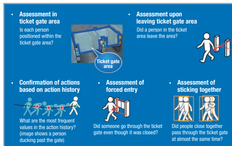
Ticket gate unauthorized passage detection system
