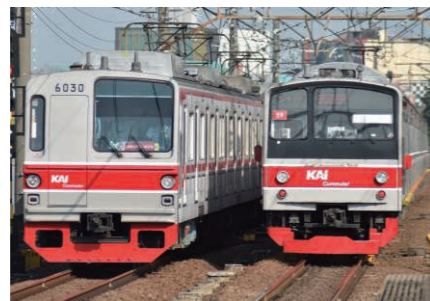
Used railcars imported from Japan (left: Former Tokyo Metro 6000 Series, right: Former JR East 205 Series)
