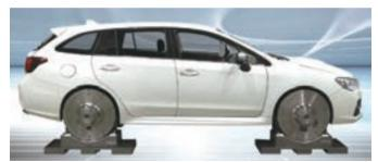
Actual vehicle test with in-wheel-well dynamo
