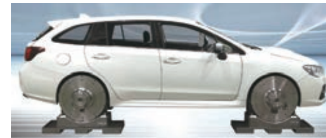
Actual vehicle test with in-wheel-well dynamo
