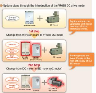
\* ED motor : Toyo Denki's permanent magnet high efficiency motor
