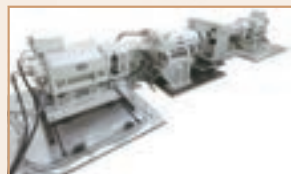
Transmission testing bench for FF vehicles
