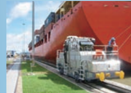
Electric towing locomotives in Panama Canal (2000)
