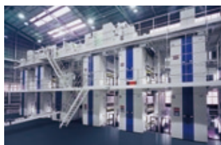
Shaftless newspaper rotary press featuring Toyo Denki components
