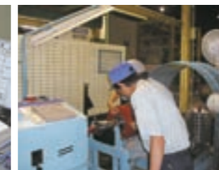
Instruction and practice of rotor dynamic balance panning work at a motor assembly workshop
