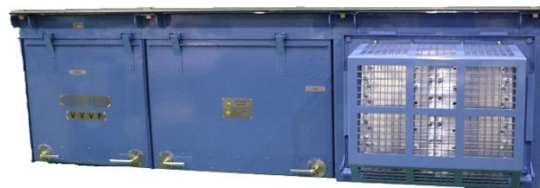
Propulsion inverters(VVVF inverter)
